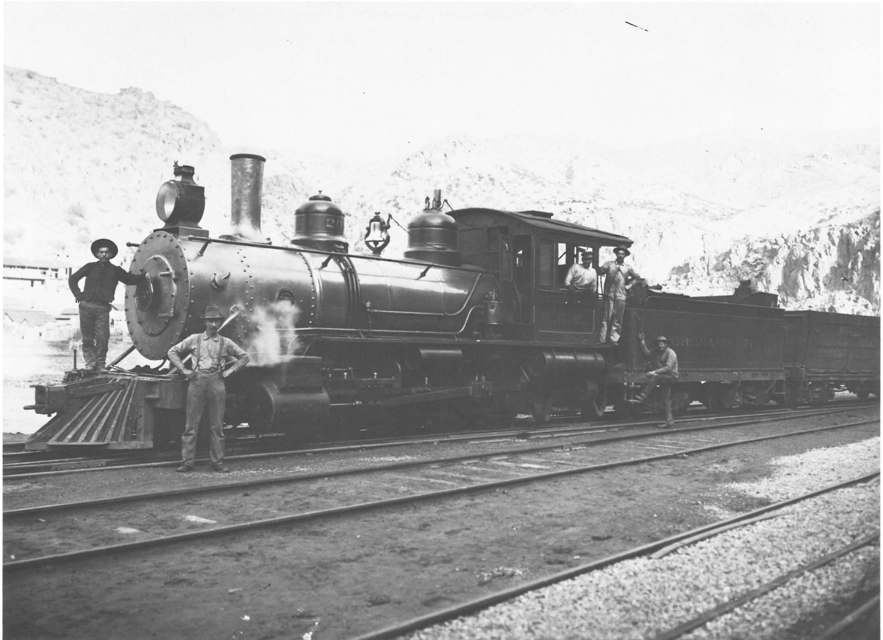
Coronado railroad engine #20 is shown parked in Clifton. The track was narrow gauge (36" between rails). Courtesy of Phelps Dodge Corporation.
